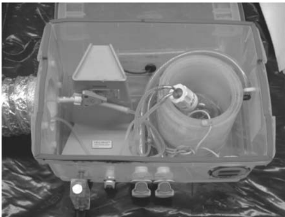
Figure 5: Imaging of the HFBR (Petersen et al., 2000). The HFBR is inserted into the magnet of the MRI system. The perfusion bottle and pin compression pump are located outside the magnet and connected to the HFBR via flexible tubing. The photograph depicts the bottle and pump. The metal vent tubing leading to the magnet is seen on the left side. Adapted from Magnetic Resonance in Medicine © 2000 (Wiley-Liss, Inc.).
